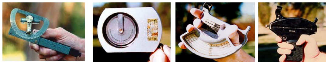
Figure 3.1. Instruments used for indirect tree height measurement (A) with left to right the Abney level, Suunto, Blume Leiss, and Haga (source: Brack and Wood 1997).
