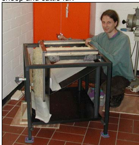
Figure 6.3. The jiggling machine ("Rüttelmaschine"); it can be used to measure attachment capacity. The comb is used to homogenise the fur and to comb the seeds into the fur.
