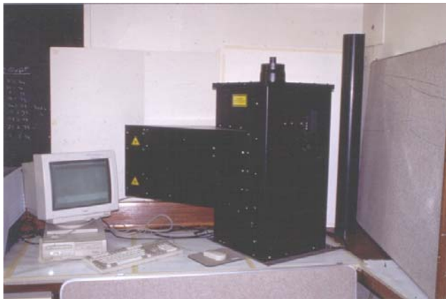
Figure 6.1. Machine for measuring terminal velocity (Photo: K. Thompson).
