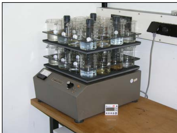
Figure 6.2. Measurement of the floating capacity of seeds using a shaking machine.
